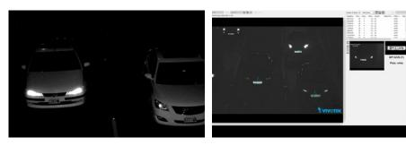
Clear Image Captured with IR Illuminators and Headlight Filter
